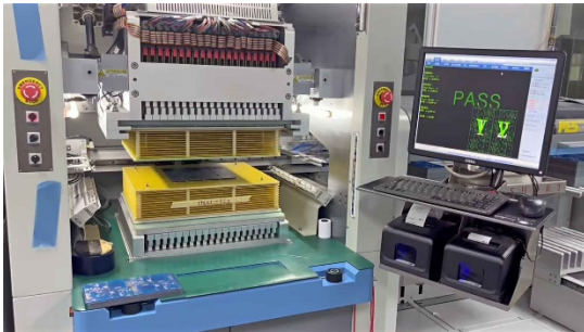
PCB Electrical Testing
